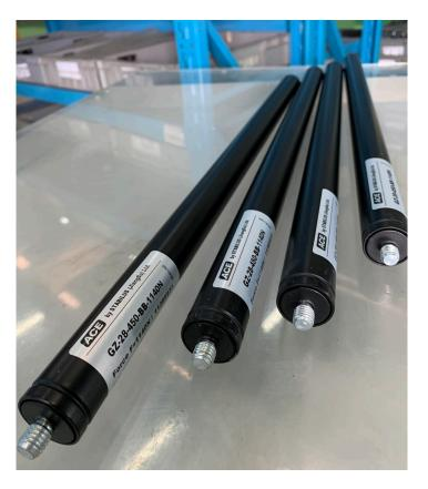
The ACE Controls' GS-28-450 pull-type gas spring provided a 270-pound traction force and low progression rate to hold the mobile X-ray device's beam arm in the final position and support raising and lowering motion.
