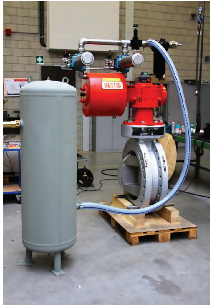
ACE industrial shock absorbers stop the piston rods inside the actuator's built-in pneumatic cylinder, which opens up the safety valves.
