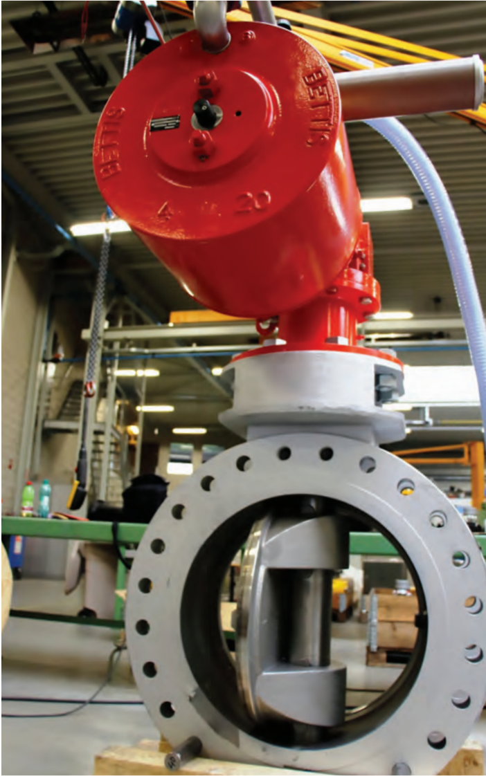
In the event of overpressure, the actuator has to open the large, 24-inch safety valve within half a second.
