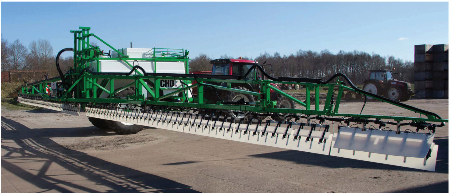
Harrie Hoeben, the brains behind the Wingsprayer, designed the machine to reduce drift during the spraying process.
